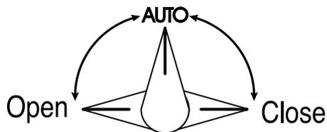
**Remember!** For controller operated irrigation, the valve lever must be in the middle (AUTO) position.
