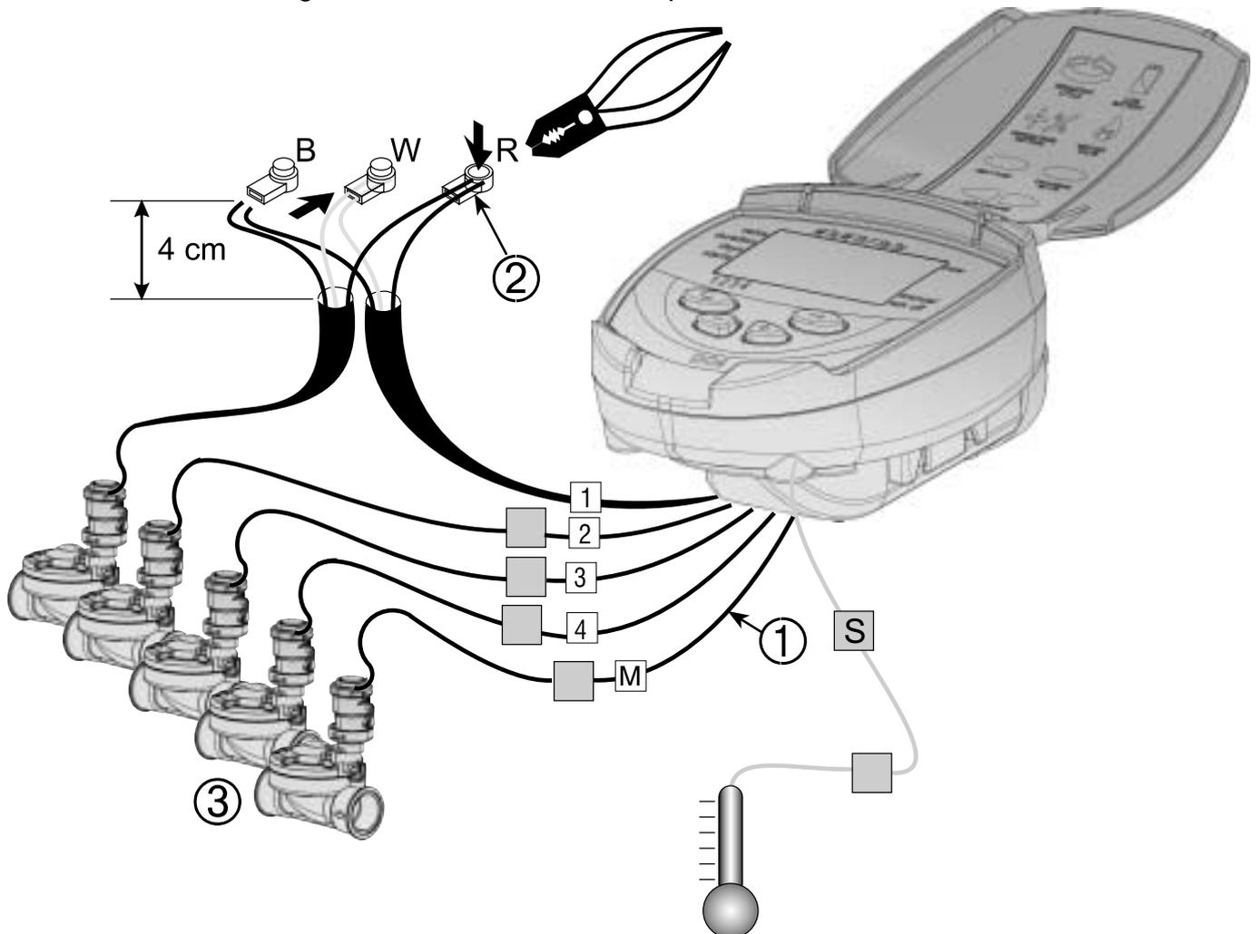
Labeled cables (1) emerge from the controller. The end of each cable is protected by a cover that must be removed prior to connecting the cable. The cables are specifically designed to connect to Galcon DC type irrigation valves and solenoids (3).
