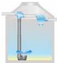
PF filter with inline siphon overflow and calmed inlet
