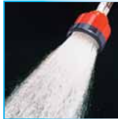
3. Seedling nozzle with micro holes. Needs filter. 42 l/min @2.7 bar
