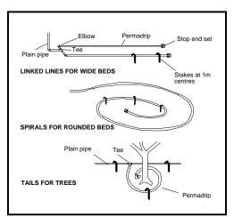
If the tap is some way from the dripline purchase a coil of 16mm polythene pipe (PA16-25M) and use the straight connector (FBK16) to join onto the dripline.
