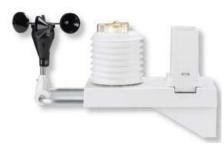
In response to the need to use water as economically as possible, the latest controllers have the ability to add an on-site weather station to the system. The controller then calculates evapo-transpiration on site and adjusts the watering times automatically, taking into account the planting type in each zone. These devices have been shown to reduce water consumption by 30%. As well as reducing water
