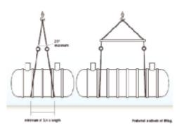
The tanks should be lifted using slings, not chains or wire ropes. For tanks longer than 5 metres, use a spreader bar or have the slings apart at least ¼ of the tank length. Do not drag the tank along the ground for any distance and avoid jarring or bumps. Do not lift with water in the tank.
