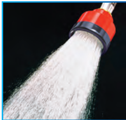
3. Seedling nozzle with micro holes. Needs filter. 34 l/min @ 2.7 bar.
