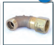
Brass Union Elbow Screws onto the top of the Quick Coupling Key to ensure the hose always points in the right direction. 1" BSPF inlet 1" BSPM outlet.
