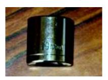
17mm long reach socket for tank brackets or 17mm ring spanner
