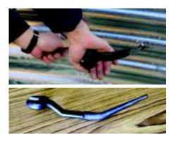
19mm socket for parabolts
