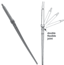
Nozzle with stake. 2 l/h @ 1 bar. Needs leads.
