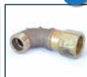
Brass Union Elbow Screws onto the top of the Quick Coupling Key to ensure the hose always points in the right direction. 1" BSPF inlet 1" BSPF outlet.
