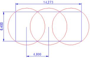
Place the first sprinkler riser in the centre of the lawn area. Connect one of the cut hose sections and then place the next riser at the end of the hose. Use the sprinkler riser with the blanking
