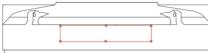
Once the weir position is marked out on the tank check once more that it is at the correct level. Drill a 10mm hole in each corner/centre and use a jigsaw, multi-cutter or pad saw to join the holes) ensure the edges are straight and ensure all swarf is removed from the edges.
