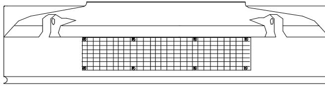
Position the mesh screen and black mesh cover centrally over the cut rectangle. Ensure the overflow edge is unrestricted (use tape to hold in place if necessary). Secure the mesh and cover to the tank using the self-tapping screws and washers provided, ensuring the cover is flat against the tank side.
