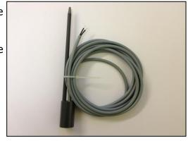
Do not use cleaning agents on the surface of the sensor as this will cause erratic misting.
